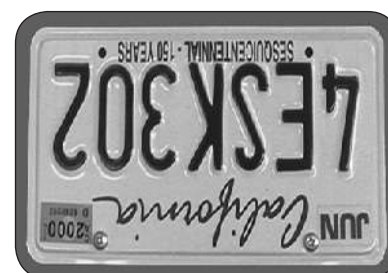
INVERTED IMAGE, AS VIEWED WITH THE EYEPIECE DIRECTLY IN TELESCOPE
