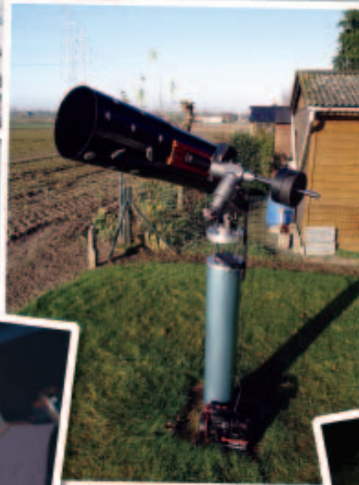
Backyard set-up featuring our C 9.25" carbon fiber tube with XLT coatings, permanent pier, goto mount and self-made dew-cap.
